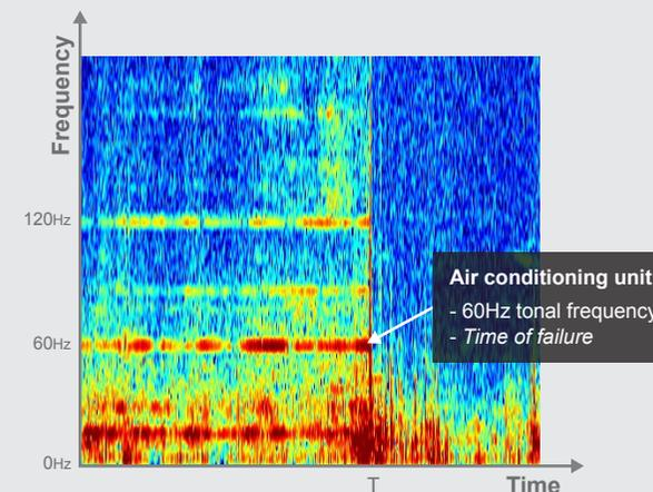
Failure of the air conditioning unit in a telecoms room at a remote block valve station had led to the shut down of critical electronic equipment due to over heating, resulting in pipeline shut down.
