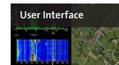
The User Interface presents the real time event data to the operator in a clear and intuitive manner where classified alerts are shown on a map display with location coordinates. By networking Interrogator Units together the system has the capability to allow an operator to monitor over 5,000km from one location and can easily be integrated with existing control systems (e.g. via OPC, Pelco etc).
